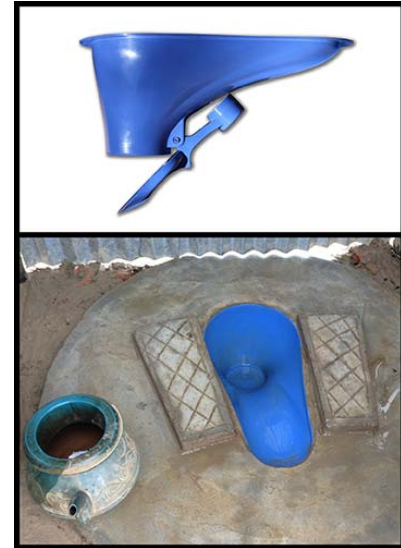
The mechanical and water seals created by this trap-door style SaTo hygienic toilet pan, invented by American Standard Brands, have improved the quality of life for residents of Bangladesh by keeping flies and insects out of open pit latrines.
